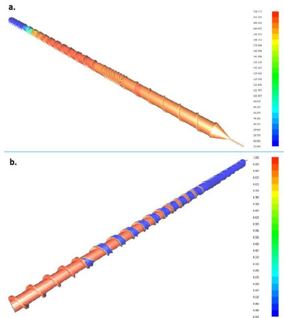
Figure 3. a) Temperature distribution, b) Solid bed distribution.
