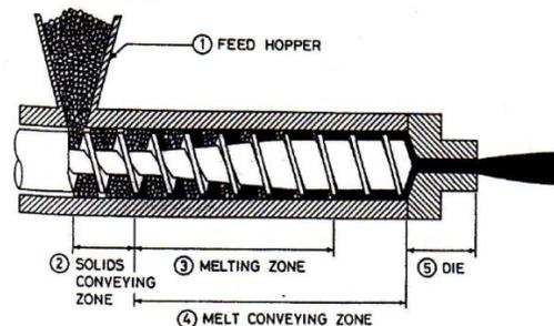
Figure 1. Schematic diagram of a plasticating extruder showing the components of the present computer model.
