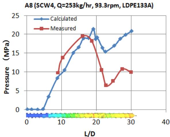
Figure 4. Pressure along axis. Measured data from ref. [12].
