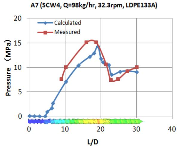
Figure 2. Pressure along axis. Measured data from ref. [12].
